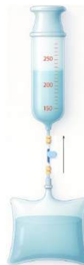
Fig. 2 Device for collecting VOCs.
